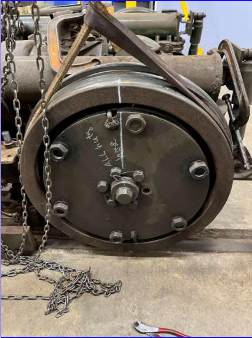
Wheel supported by sling after nuts and bolts are loosened; note the index line
