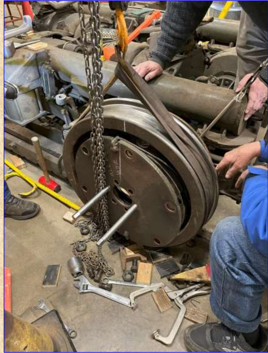
7/8"-14 UNF threaded guide rods maintain wheel component registry
