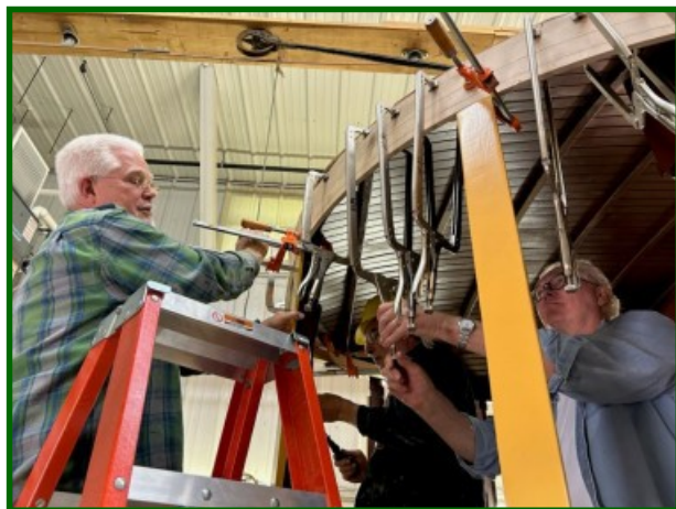
Old woodworker's saying: you can't have too many wood clamps. From the steamer to the streetcar, Howie Melco, Michael Kimitich and Carl Floren quickly clamp the header board in place after it was taken out of the wood steamer and clamp it in place so it will retain the curvature on the end of No. 265. (Karen Kertzman photo)
