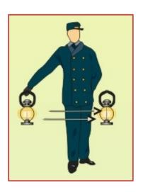
**3. REVERSE**Made in relation to the operator's position - i.e. put the reverser handle in the reverse position. Swung in a circle.
