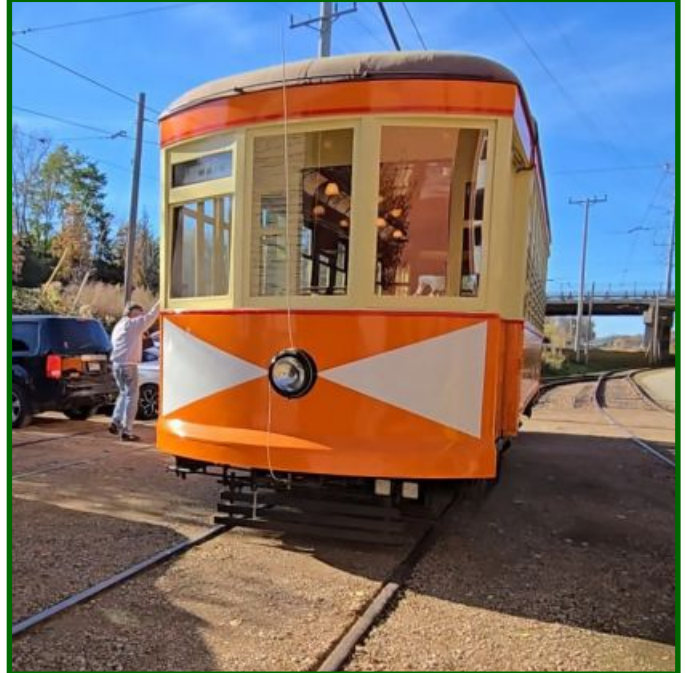
Carl Floren will shortly operate Mississippi Valley Public Service (Winona lines) No. 10 on ESL's track for further testing following the machining and adjusting of the brake heads and shoes. (Dick Zawacki photo)
