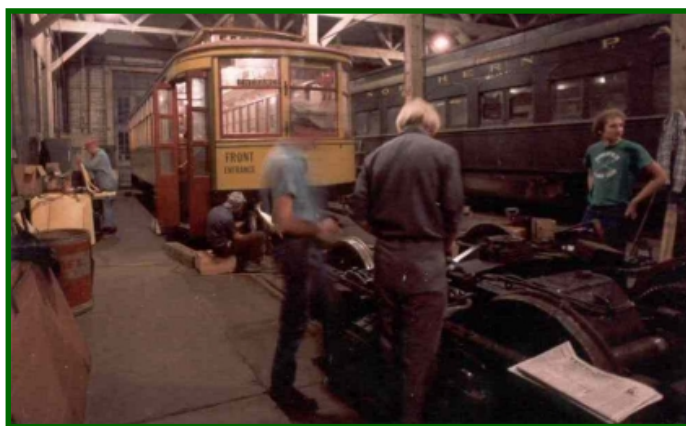
Here are two photos of the work on DSR No. 265 taken in 1973 and 1974 at the ex-NPRR Como Shops. The photo of the left shows No. 265 and the temporary shop truck in front that came off the TCRT electric locomotive. The rear truck is one of the Chicago "EL" trucks and it still has the 3d rail shoe on it! On the right No. 265 is nearly ready to go to CHSL. The guys on the right are doing some work on one the Chicago "EL" trucks.
