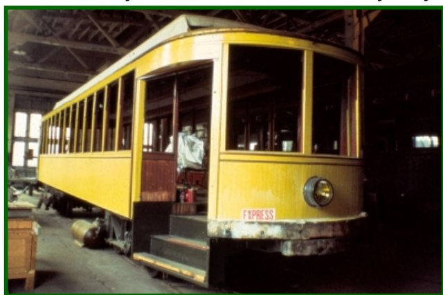
Here are two photos of the work on DSR No. 265 taken in 1973 and 1974 at the ex-NPRR Como Shops. The photo of the left shows No. 265 and the temporary shop truck in front that came off the TCRT electric locomotive. The rear truck is one of the Chicago "EL" trucks and it still has the 3d rail shoe on it! On the right No. 265 is nearly ready to go to CHSL. The guys on the right are doing some work on one the Chicago "EL" trucks.
