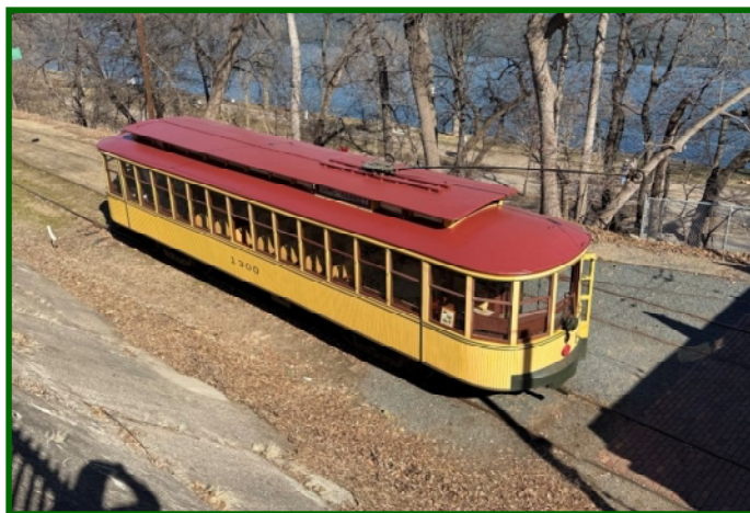
Looking Good. All of TCRT's standard streetcars had roofs of stretched canvas painted in the familiar red color. Needless to say, these had to be replaced periodically, with cleaning and painting in between major overhauls at Snelling Shops. Karl Jones led a CHSL team to paint the roof so it'll last for a few more years. (Jerry Betz photo)
