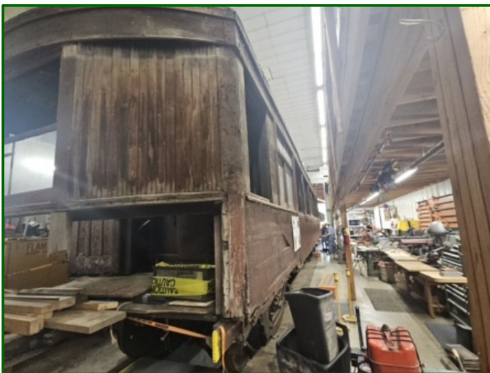
Close quarters, eh? While Mesaba No. 10 is in the shop, the goal is not to make the classic interurban operational, at least not yet. Structural and cosmetic work will be done to make the car accessible to the public (the rear platform is basically gone) and somewhat pleasing to look at. This is the Motorman's end of No. 10. (Karen Kertzman photo)
