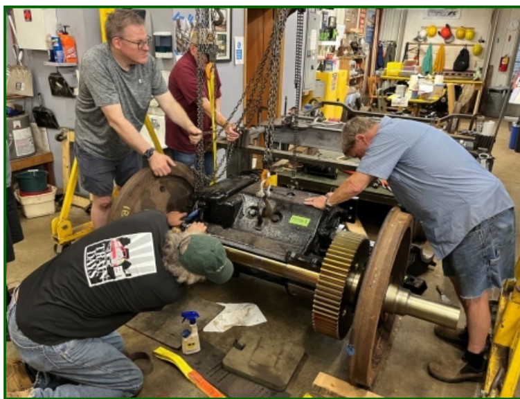
We reached a critical juncture in the No. 1239 truck project: fitting both bronze suspension bearings (aka, "brasses") to the motor journals and axles. A number of folks participated in wrestling the traction motor into position relative to the wheelset. Standing, from left are Jerry Betz , John Prestholdt and Tom Schramm . Rob Mangels has his back turned as he checks fitment. (Dennis Stephens photo)
