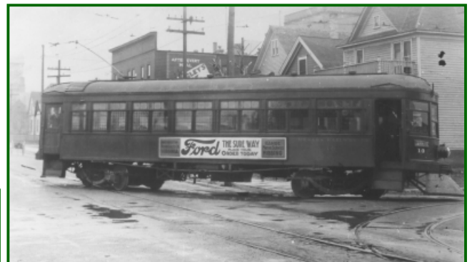
Passenger motor car 10 turning on the Virginia [Minnesota] wye. The pilot has been covered with steel plate for snow plowing purposes, and advertising revenue has been solicited from the competition.
