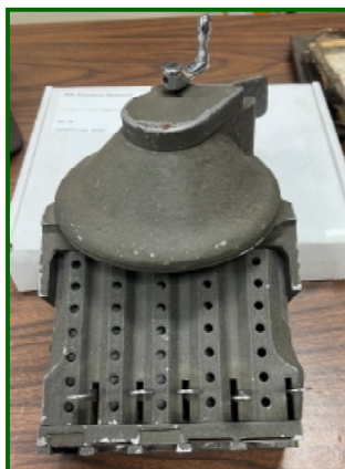
The rack for the Kessler Changer (St Louis Car Co photo)
